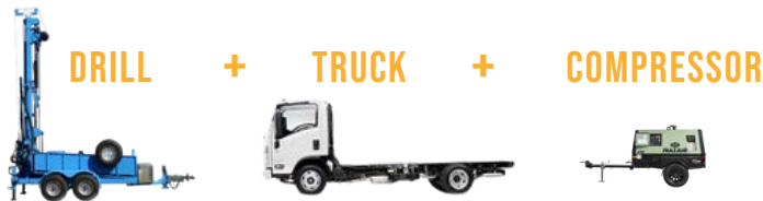
The new rig consists of a heavily modified LS300T+ drill from Little Beaver and LoneStar Drills, mounted on a 4WD Isuzu truck with a hard-mounted compressor.
